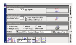
it would be necessary in order to convert the whole text to an attribute, to convert these single letter-geometry elements to one text element. Nevertheless, the existing text must be arranged within the tolerance to be entered (distance from horizontal).
