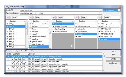
This application helps to find layers, to switch visibility (freeze/thaw) and to create layers not already existing in the drawing.
