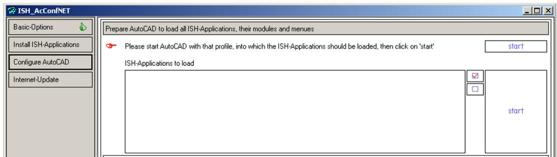
Start AutoCAD and press 'start' in the first line.
