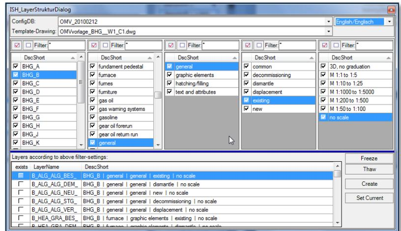
This application helps to find layers, to switch visibility (freeze/thaw) and to create layers not already existing in the drawing.
